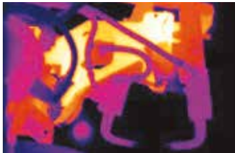
Hot spot in welding robot
